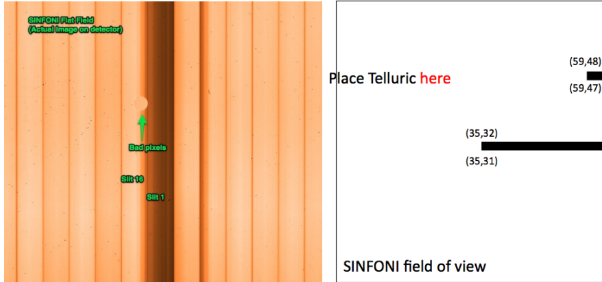
Figure 8: Left: This is a SINFONI Flat Field image. The disc of bad pixels near the centre of the detector falls on slit #16, which crosses the centre of the field of view of SINFONI. Right: This is the reconstructed FOV of SINFONI, showing the location of the blind spots. Slit #16 corresponds to y=31 and 32 . Slit #24 corresponds on y=47 and 48 .
