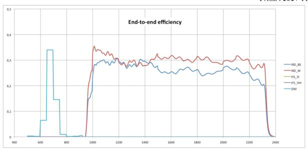
Figure 35: Transmission (as above) in IRDIS alone configuration where all the NIR light is sent to IRDIS.
