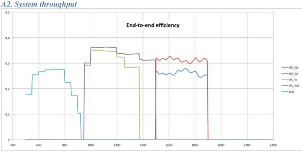
Figure 33: Transmission from SPHERE entrance to the science detectors, including the detector efficiency, assuming i) no coronagraph, ii) ZIMPOL path goes through the GREY beamsplitter (80% to ZIMPOL), and iii) the H dichroic separating the flux between IFS (up to 1450 nm) and IRDIS. Note that IRDIS cannot observe in K band in this setup.
