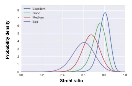
Figure 28 Probability distribution of the Strehl at H-band for stars of R magnitude between 9 and 11 with IRDIS or IFS in the proposed new categories. All distributions have been normalized to an integral of 1.
