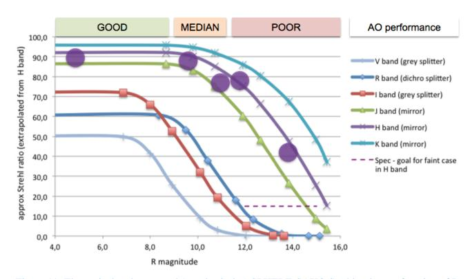
Figure 11: Theoretical and measured (purple circles) SPHERE-SAXO Strehl ratio as a function of R magnitude for good seeing conditions and different wavelength ranges from V to K (see Table 11 and Table 12 for details).
