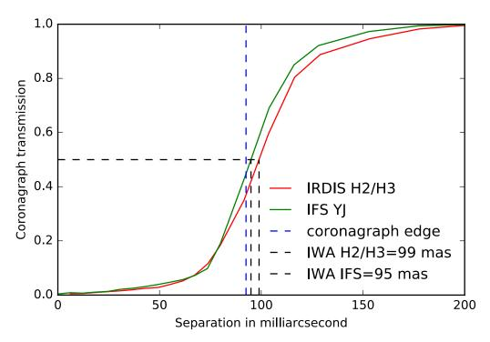
Figure 43 Transmission profile for the N\_ALC\_JYH\_S coronagraph
