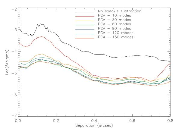
Figure 18: IFS  $5\sigma$  sensitivity on Iota Sgr as function of angular separation, for different principal components retained in the speckle subtraction using both spectral and temporal diversity (ADI).
