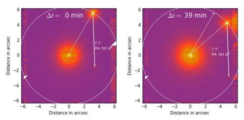
Figure 38: IRDIS ghost appears when there is a bright source on upper right corner of detector.
