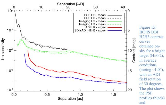
coronagraphic profiles (green) in the H2 and H3 filters, the  $1\sigma$  contrast curve for ADI on the H2 data (red), and the  $1\sigma$  contrast curve for SDI+ADI on the H2 and H3 data. For the ADI and SDI+ADI analysis, the algorithm throughput is taken into account and compensated, assuming a T8 spectral-type for the planet in SDI.
