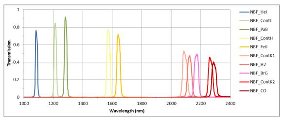
Figure 41: IRDIS NB filters.
