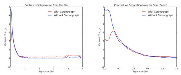
Figure 13: Contrast obtained with and without the use of the coronograph. Contrast is in H band magnitudes. Right: zoom for separations less than 1". Note that the separation shown here is in arcsec, and not in AU.
