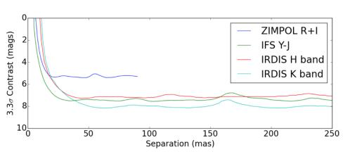
Figure 25: SAM\_7H contrast limits for the detection of companions in various bands from the test data (July 2015). Each dataset consisted of approximately 1hr in execution time, including time for observations of calibrator stars. This was obtained on the F6 star HD142527 with R=8.3, J=6.5, H=5.7, K=4.98 with a seeing ~0.6-0.8". HIP113246 and HD169319 were used as calibrator stars (Cheetham et al., in prep.).
