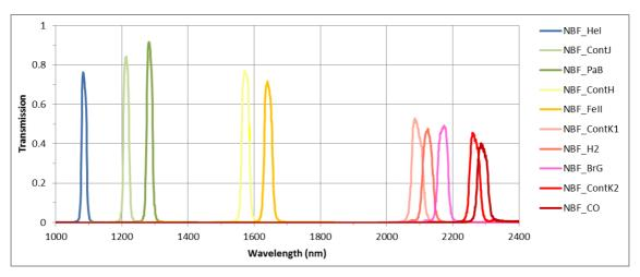
Figure 31: IRDIS NB filters.
