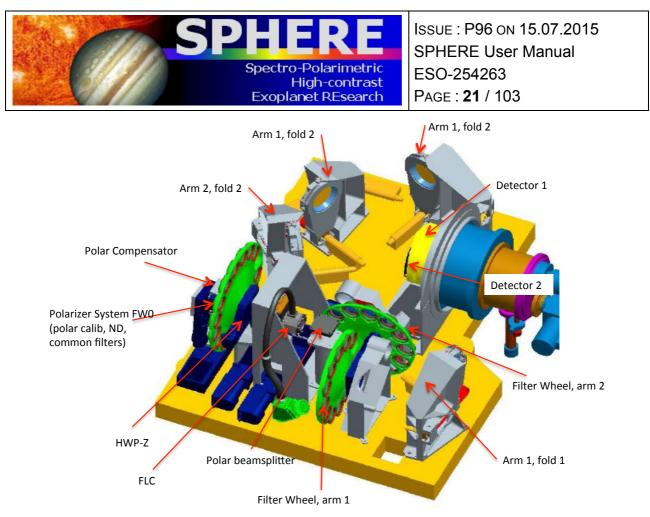
Figure 7: ZIMPOL schematic view showing the main elements of this visible polarimeter, from polarization compensator, common filter wheel, Ferroelectric Liquid Crystal (FLC) modulator to the splitter, filter wheels 1 and 2, and the two detectors.
