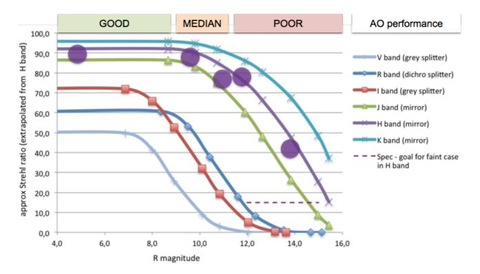
Figure 10: Theoretical and measured (purple circles) SPHERE-SAXO Strehl ratio as a function of R magnitude for good seeing conditions and different wavelength ranges from V to K (see Table 997 and Table 10108 for details).
