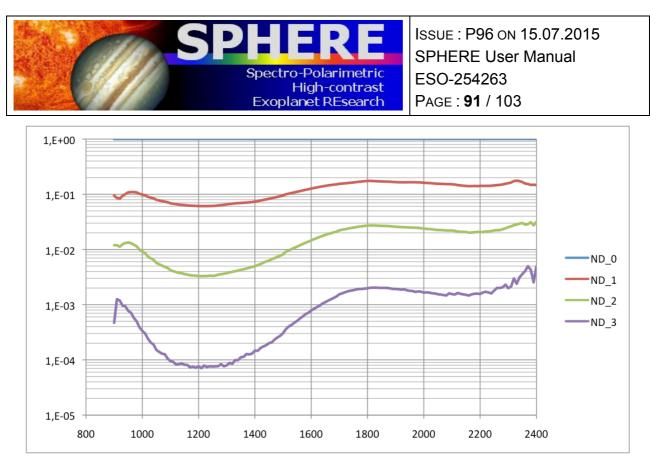
Figure 27: Transmission CPI NIR densities as a function of wavelength (nm).
