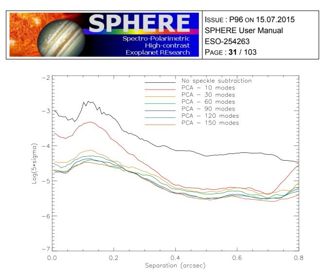
Figure 16: IFS 5σ sensitivity on lota Sgr as function of angular separation, for different principal components retained in the speckle subtraction using both spectral and temporal diversity (ADI).
