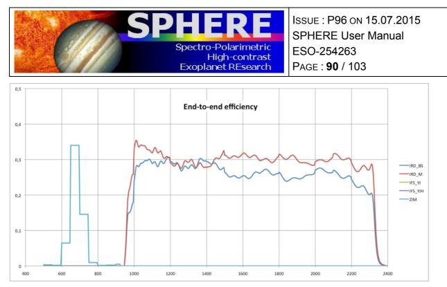
Figure 26: Transmission (as above) in IRDIS alone configuration where all the NIR light is sent to IRDIS.
