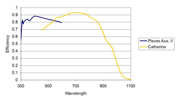
Figure 8: UVB/VIS detector efficiency.
