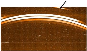
Figure 20: Leak in the K-band blocking filters.
