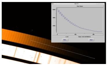
Figure 21: 0.6"JH slit, some low level interferences are visible in the reddest part of the last order.
