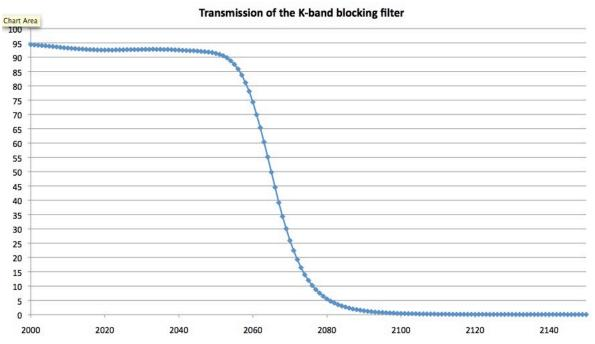
Figure 10: Transmission curve of the K-band blocking filter.
