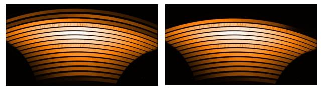
Figure 11: Flatfield frames for the normal 0.9" NIR slit (left) and for the 0.9" with K-band blocking filter (right). The last orders are cut with the K-band blocking filter.
