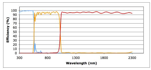
Figure 6: The combined efficiency of the two dichroic beam splitters. Reflection on dichroic 1 (blue); transmission through dichroic 1 and reflection on dichroic 2 (orange); transmission through dichroics 1 and 2 (red).
