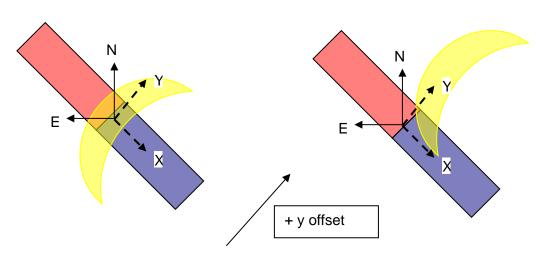
Figure 35: The offset with PA= +45 degrees shows a positive offset in y axis. The object moves in +y, while the slit moves in the -y axis.
