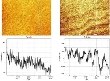
Figure 30: Fringing in r\_prime and z\_prime. The most affected filters are r\_prime, i\_prime, z\_prime, and I. The peak-to-peak amplitudes range from 2% in r\_prime to 4% in z\_prime.
