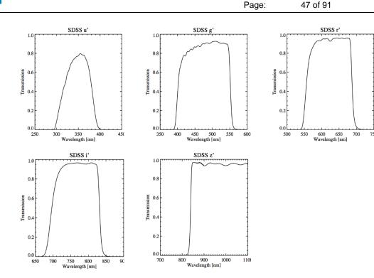
Figure 27: A&G camera filter curves.
