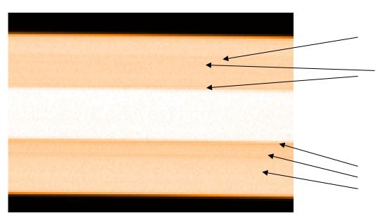
Figure 23: Example of small irregularities of the edges of the IFU mirrors in the NIR arm.
