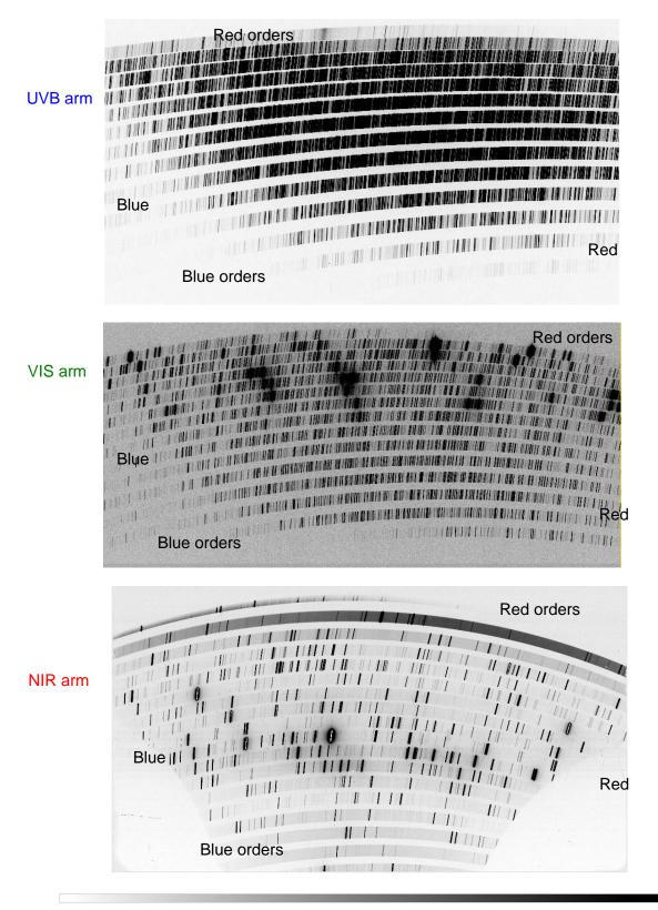
Figure 17: Example of UVB (top), VIS (middle), and NIR (bottom) calibration frames. Strong order curvature and varying slit tilt and scale are clearly visible. Note the higher thermal background at longer wavelengths for the NIR arm, in particular in the 11th order (K band).
