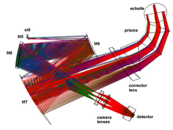
Figure 9: The NIR spectrograph optical layout.
