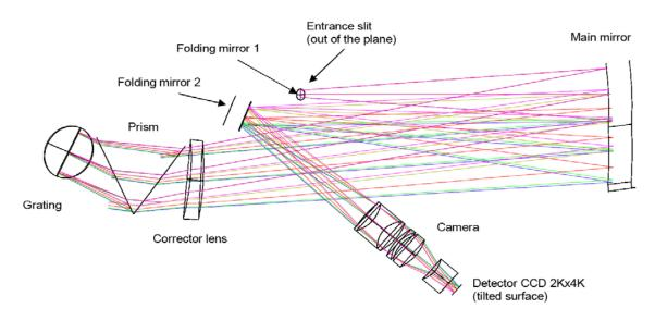
Figure 7: The UVB spectrograph optical layout.
