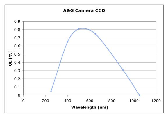
Figure 26: A&G TCCD quantum efficiency curve.
