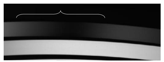
Figure 15: SLIT UVB QTH flat field. The dip due to the first dichroic is visible in the top order.
