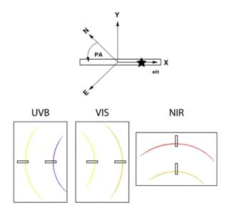
Figure 32: Slit coordinate system and relation between object position in the slit and position on the spectrum. An object at positive x (black star top panel) produces spectra placed as illustrated in the
