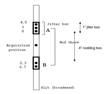
Figure 24: Conventions used for a nodding of 4" along the slit. The sequence illustrated here corresponds to 4 cycles (8 exposures, ABBAABBA) with a jitter box of 1".
