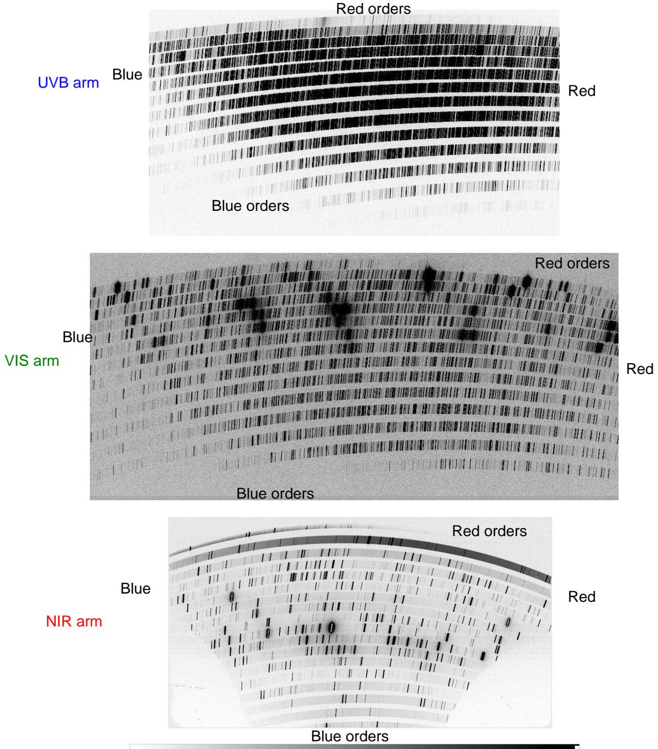
Figure 10: example of **UVB** (top), **VIS** (middle) and **NIR** (bottom) calibration frames. Strong order curvature and varying slit tilt and scale are clearly visible. Note for the **NIR** arm the higher thermal background in longer wavelength. This is specially the case in the 11<sup>th</sup> order that corresponds to the K band.
