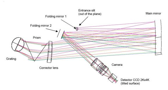
Figure 7: The UVB spectrograph optical layout
