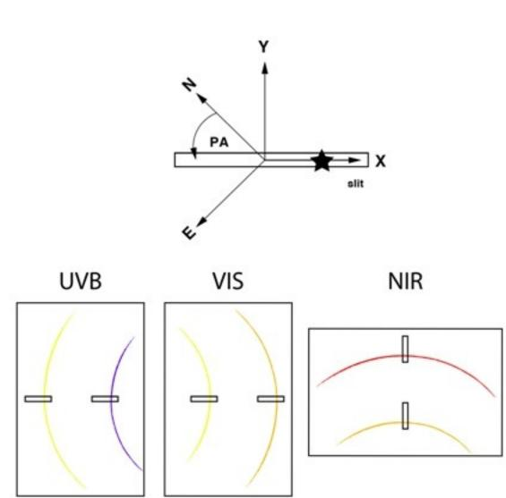
Figure 19: The slit coordinate system and correspondence between object position in the slit and position on the spectrum for each arm. An object at positive x (black star top panel) produces spectra placed as illustrated in the bottom panels. NOTE: a positive offset in the x or y direction will move the object in direction of +x and +y axis.
