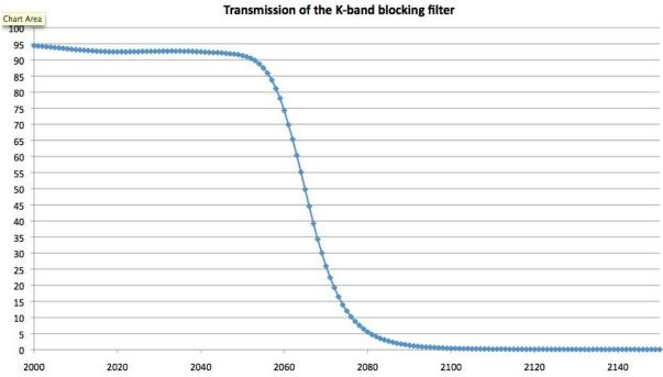
Below is the transmission curve of the K-band blocking filter.
