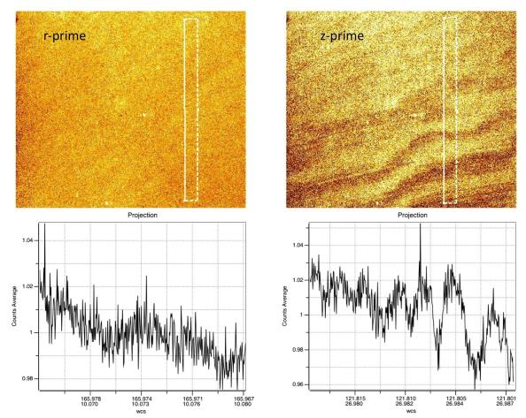
Fig. 7bis: Fringing maps in r' and z'. The cuts in the bottom show the amplitude peak to peak of the fringes.
