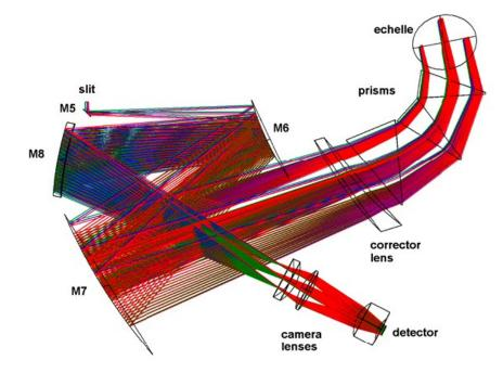
Figure 8: The NIR spectrograph optical layout.
