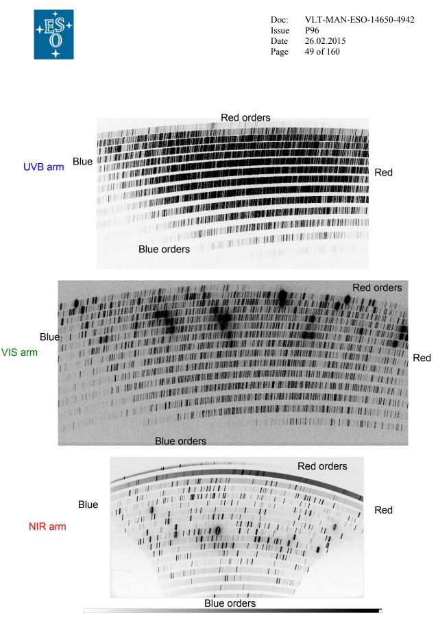
Figure 10: example of UVB (top), VIS (middle) and NIR (bottom) calibration frames. Strong order curvature and varying slit tilt and scale are clearly visible. Note for the NIR arm the higher thermal background in longer wavelength. This is specially the case in the 11<sup>th</sup> order that corresponds to the K band.
