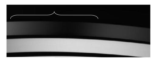
Figure 11: SLIT UVB QTH flat field, UVB arm, the dip due to the first dichroic is easily visible in the top order.
