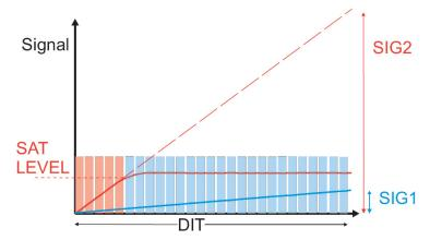
Figure 9: Saturation threshold for nondestructive sampling and extrapolation of detector signal for high flux levels. For pixels with high flux (red) only readout values below SATLEVEL (orange rectangles) are taken into account in the calculation of the slope and values written in the FITS files are extrapolated to the full DIT (SIG2). For low flux pixels (blue) all nondestructive readouts are used (light blue rectangles). Figure courtesy of Finger at al. (2008).
