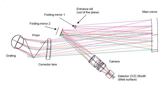
Figure 7: The UVB spectrograph optical layout
