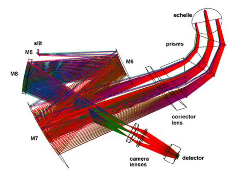
Figure 8: The NIR spectrograph optical layout.
