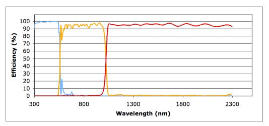
Figure 6: The combined efficiency of the two dichroic beam splitters. *In blue*: reflection on dichroic 1; *in orange*: transmission through dichroic 1 and reflection on dichroic 2; *in red*: transmission through dichroics 1 & 2.
