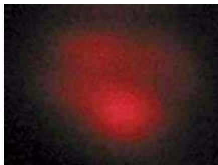
Figure 22 IR spot after SHG with PPKTP waveguide. The spot was made visible on an IR viewing card. The picture has been taken 6cm after the chip and the spot is a bit smaller than 2cm. The faint details are not visible on this picture.
