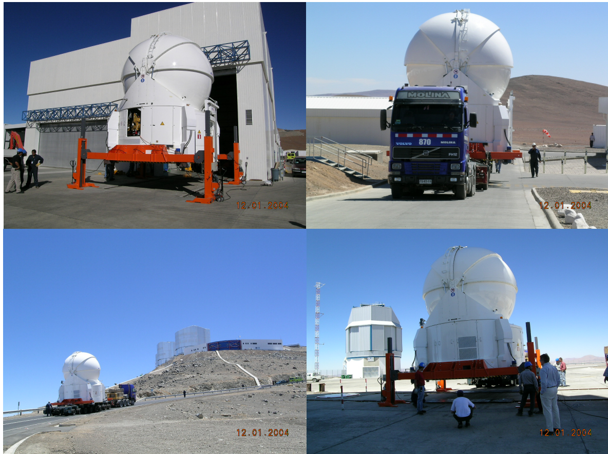
Figure 4: The first Auxiliary Telescope is transported from the MMB to the Observatory Top on 12/1/04. The fully integrated AT weighting 33 tons is lifted with a specially-designed tool and is loaded onto a hydraulic trailer. (Photo: R. Tamai)
