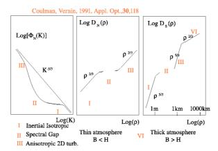
Figure 9. Behavior of the phase structure function  $D_S(\rho)$  with baseline  $\rho$
