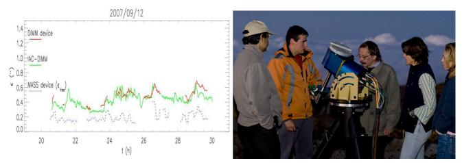
Figure 4. Left: Comparison of seeings measured with the reference IAC-DIMM with the ELT-DIMM and the MASS. Both dimms compares very well and, as MASS is insensitive to ground layer turbulence, it gives better seeing than the dimms. Right: People who participated to ORM DIMM calibration campaign: Z. Benkhaldoun, H. Vazquez, V. Kornilov, Casiana and A. Varela.
