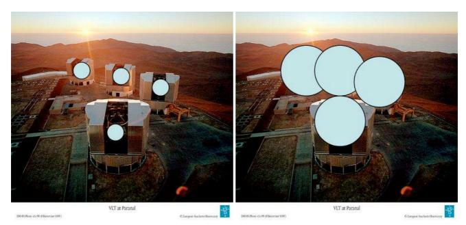
Figure 10. Left: Seen from a single star, one can probe four 8 m wave front. Right: Seen from many stars within a 8 arcmin field of view, at 45 degrees from zenith and for a layer moving at 10 km altitude, one can notice that each pupil is larger and they begin to overlap, allowing a full reconstruction of the wavefront over  $\sim 100$  m.
