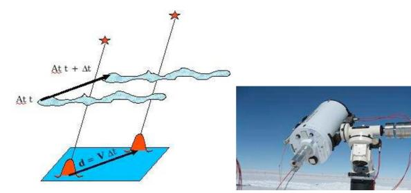
Figure 8. Left: SSS principle. Right: SSS prototype in operation at Dome C. The same instrument is installed at "Observatoire de la Côte d'Azur" in the framework of ELT-DS.
