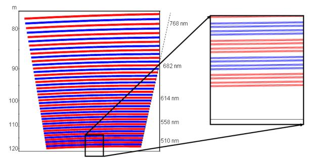
Figure 2. Spectral format of the red arm of ESPRESSO. A similar format with shorter orders is available for the blue arm. The zoom on the right side shows the four slices of each order (2 for the target and 2 for the reference fiber). Distinct orders are distinguished by different colors.
