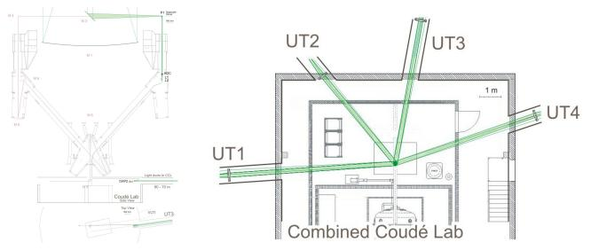
Figure 3. Left: Optical path from the M3 of an Unit Telescope (UT) of the VLT to the entrance of the light tunnels. Right: Incoherent recombination of the light beams from the four UTs in the Combined Coudé Laboratory, before being injected into a single spectrograph fiber.
