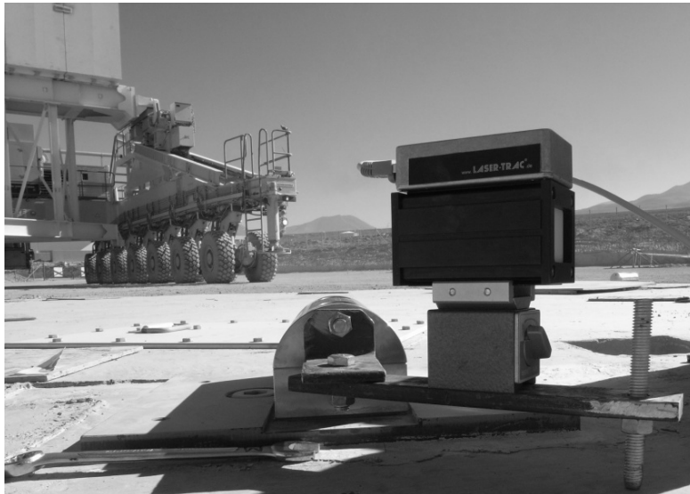
5 Laser Detector CCD installed on Interface block
