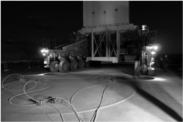
8 Antenna dummy before lowering down on foundation with Sensors installed
