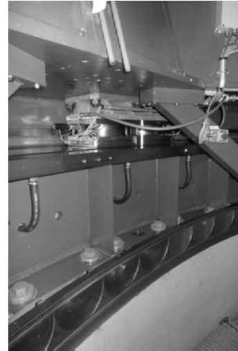
9 Telescope Azimuth Track with Hydrostatic Bearing
