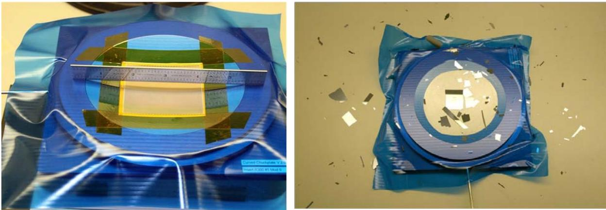
Figure 9. (Left) Successful spherical curvature before (Right) self destruction due to stress
