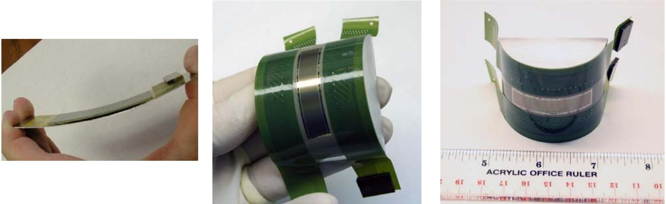
Figure 3. (Left) Early ITL cylindrically curved 2k x 4k CCD with low curvature radius, (Middle and Right) Cylindrical STA0520 2688 x 512 CCD with  $\sim 25$  mm radius of curvature
