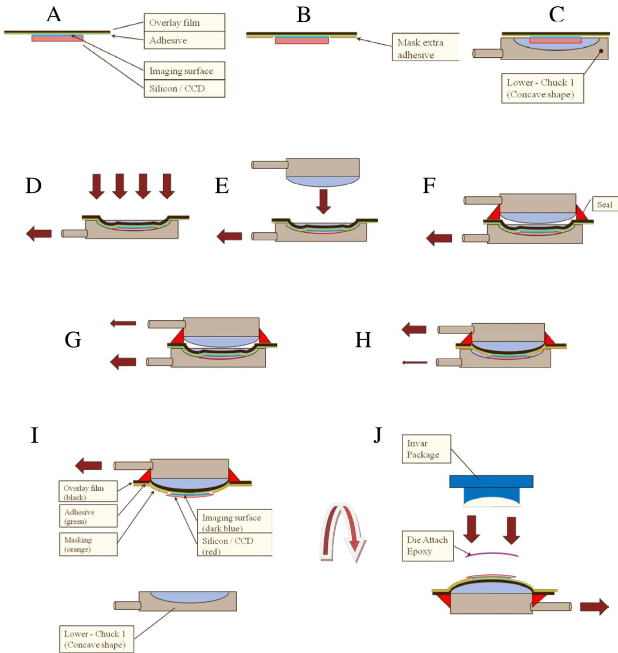
Figure 6. "Double Vacuum Process" illustrated in basic steps A to J in simplified form (compare Figure 5 and the text of this section for explanation)
