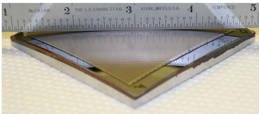
Figure 4. Photograph of convex curved frontside-illuminated ITL detector (thickness  $500\ \mu\text{m}$ ) with size of  $60 \times 60\ \text{mm}^2$ , curvature radius  $\sim 500$  mm.
