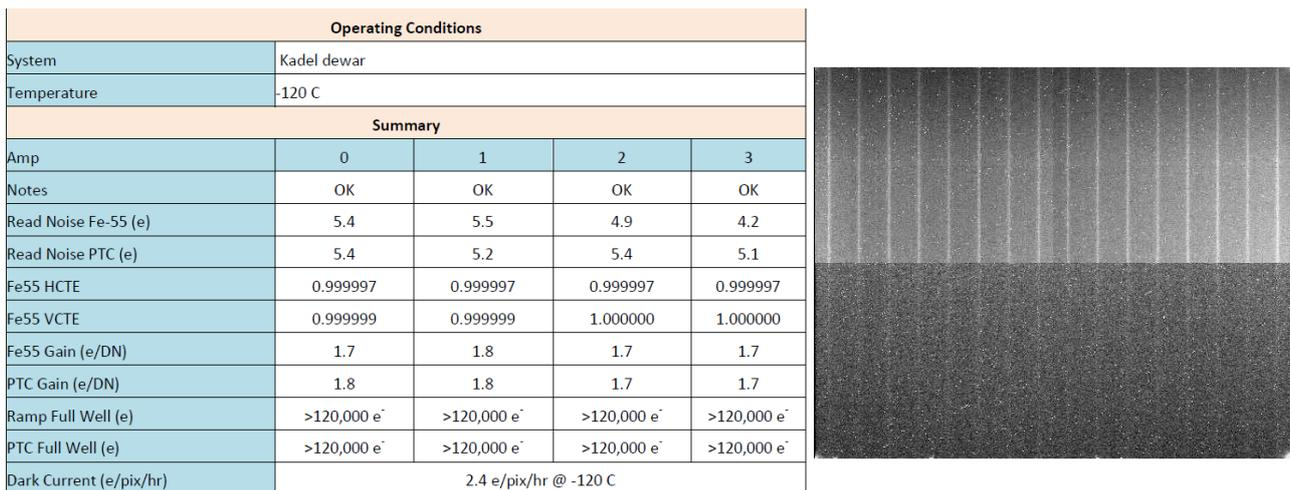
Figure 13. (Left) Exemplary measurement data of main CCD parameters after curvature (Right) Exemplary dark exposure of 600 sec. at -120°C of curved device. Visible stripe patterns are independent of curvature process (metal strapping for high speed clocking on STA2900 devices)
