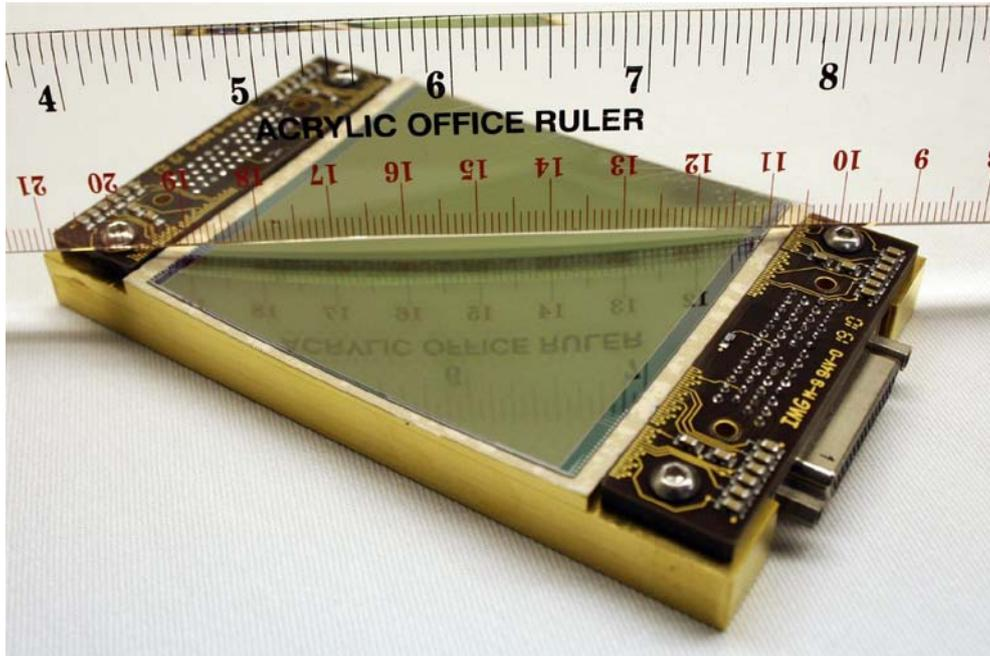
Figure 8. One of three working curved frontside-illuminated devices with 4k x 4k, 15  $\mu\text{m}$  pixelsize, 60 x 60  $\text{mm}^2$ , curvature radius  $\sim$  500 mm in two dimensions. Starting point was an STA 2900 device.
