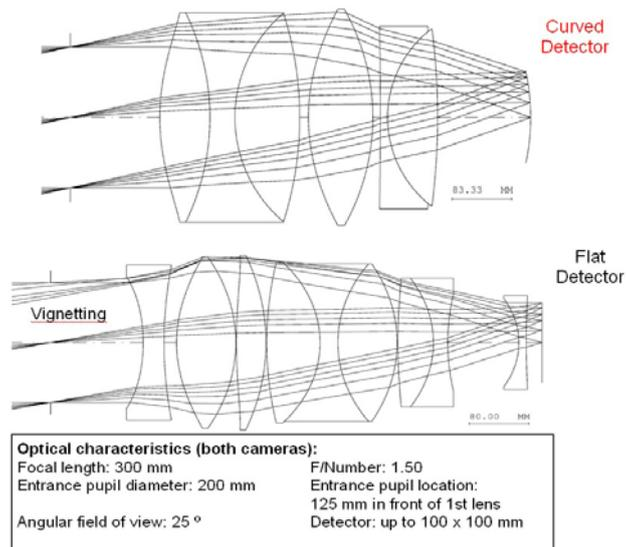
Figure 1. Comparison of optical design with curved detector in two dimensions (top) and flat detector (bottom). The optical characteristics of both cameras are given in the table.
