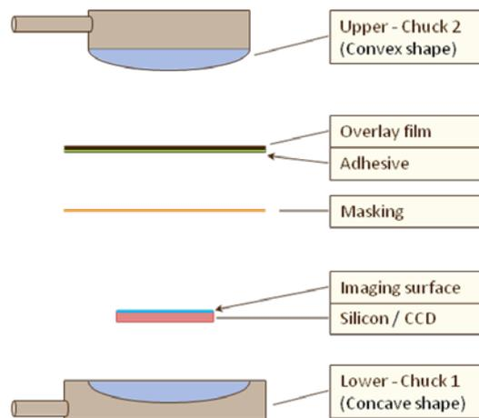
Figure 5. Individual components of “Double Vacuum Curving Process”
