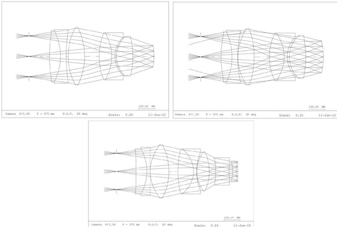
Figure 2. Comparison of optical design with curved detector in two dimensions (top two) for 20 and 30 degree field, and flat detector (bottom) with lower image quality
