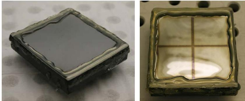
Figure 14. (Left) The curved mosaic part mounted backside-upward onto the curved, acid-resistant ceramic. An expedient wax border protects critical edges from attack. (Right) The successfully etched part. The dark lines relate to the space between the dies.
