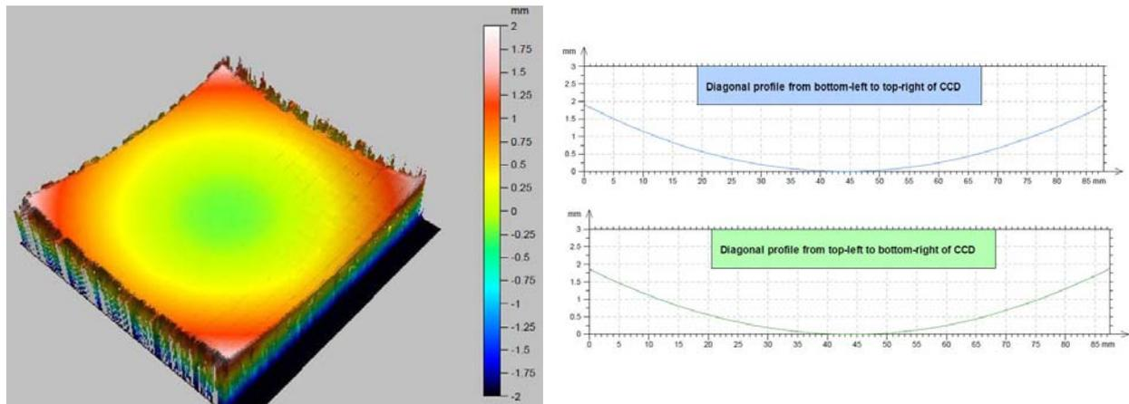
Figure 12. (Left) 3D surface profile (Right) Curvature radius measurements across device
