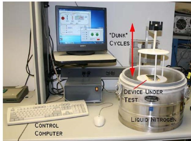
Figure 11. Setup for cryogenic stress testing of curved device
