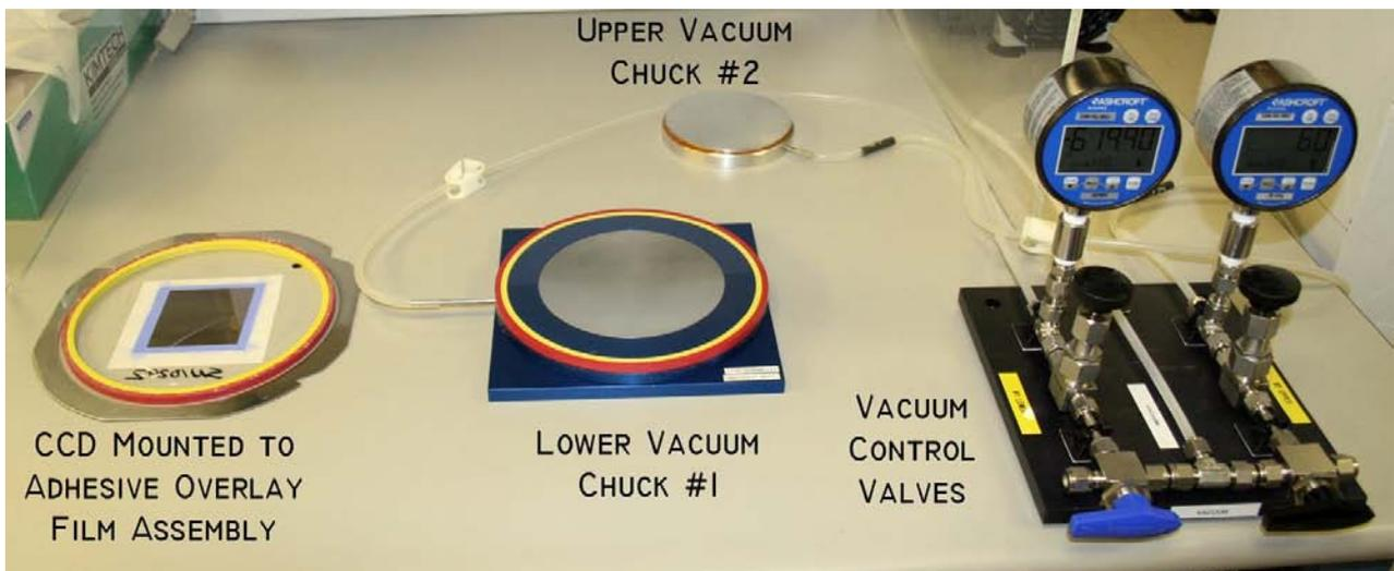
Figure 7. The process hardware to curve devices (compare Figures 5 and 6 for the different parts and process steps)
