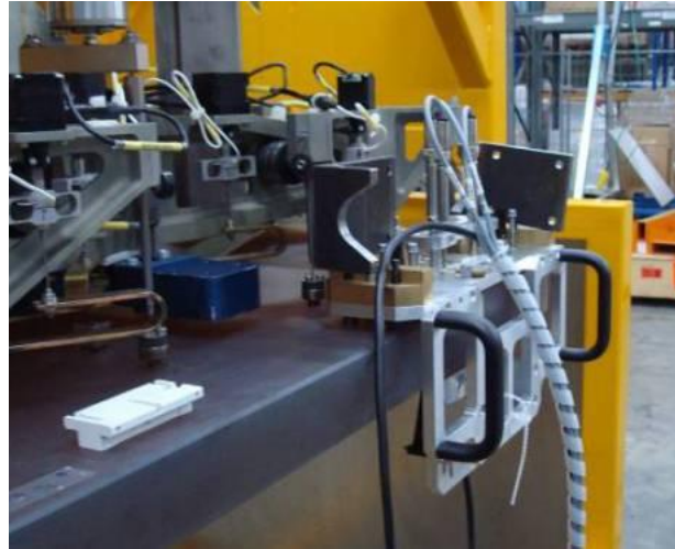
Figure 8. First generation Edge Sensor alignment during integration (left: measurement principle, right: tooling)
