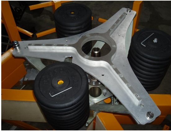
Figure 3. Fixed Frame alignment tool without separation of lateral and axial constraints
