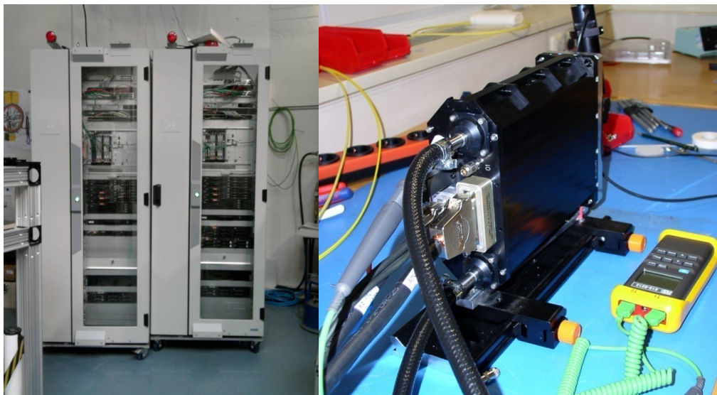
Figure 4: The left picture shows the two cabinets hosting the GRAAL and GALACSI SPARTA real time computers as well as the servers required to control the tip-tilt and WFS cameras. These host the real time box, servers for off-line processing and switches for fast communication and connection to the networks. The right side picture shows one instance of the wavefront sensor camera in its compact housing. The latter is sealed and flushed with dry nitrogen. The detector cooling is ensured via a Peltier cooler (see water pipes connecting at the back).
