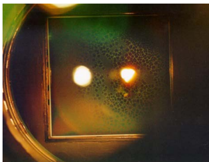
Figure 2. Contamination of 2x2k Tektronix backside thinned CCD detector with grease shows crocodile pattern
