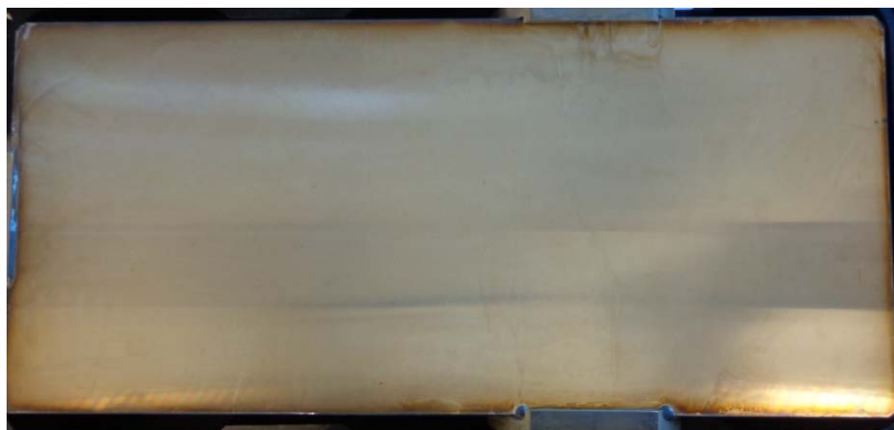
Figure 3. WFOV optical CCD mosaic with typical cryostat contamination (water vapor monomolecular layer and maybe some hydrocarbons)
