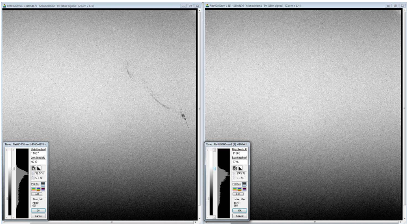
Figure 11. Flat-field of detector before (left) and after (right) vapor cleaning
