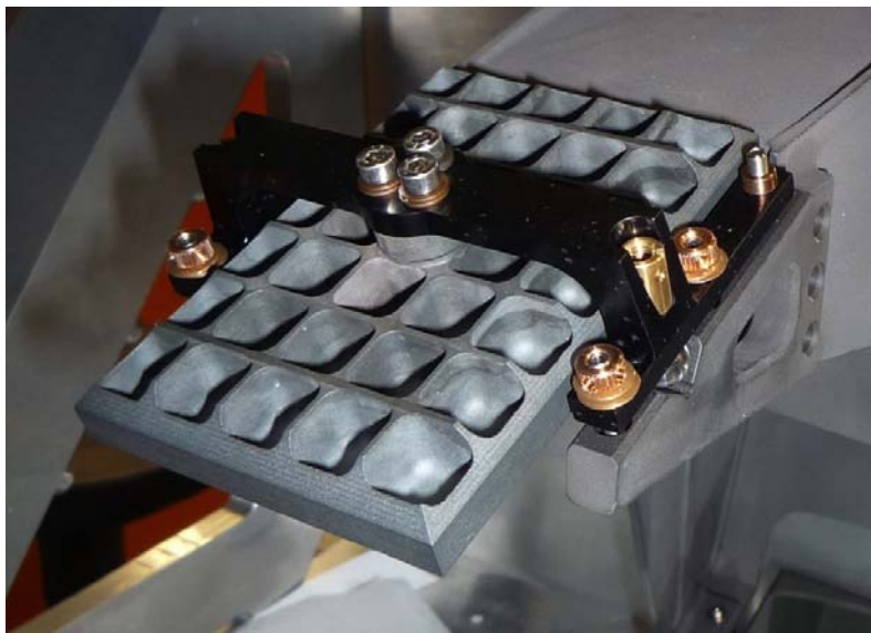
Figure 6. Attachment of the Pickup mirror to the bridge for its assembly. On the top right hand side it is shown the detail for the mounting fixation of the mirror to the bridge and on the top left the detail of the invar interface which decouples the attachment interface from the optical surface. The photo at the bottom shows the assembled pickup mirror; identical principle is used for all mirrors in the new supporting arm.
