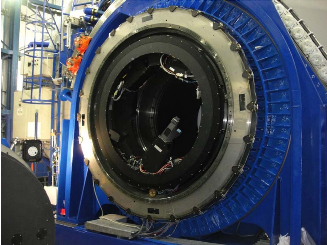
Figure 15. The new supporting arm installed on the sensor arm at the Nasmyth adapter rotator of UT4
