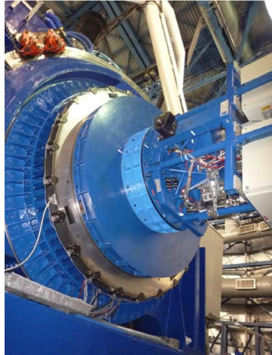
Figure 16. On the left it is shown the extension flange verification at the manufacturer premises. On the right the ~1.2m diameter spacer to install the VLT test camera at the proper focal plane position (extended by 250mm) at the Nasmyth focus.
