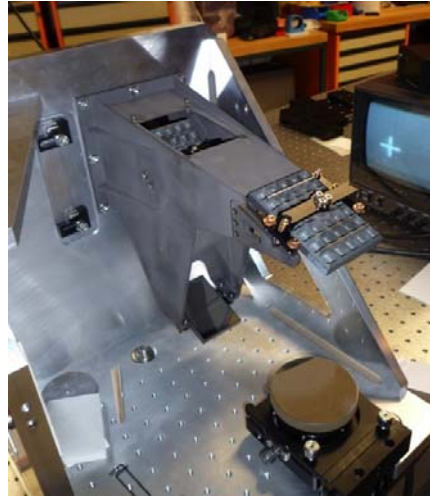
Figure 10. Partially integrated new supporting arm on the integration stand.
