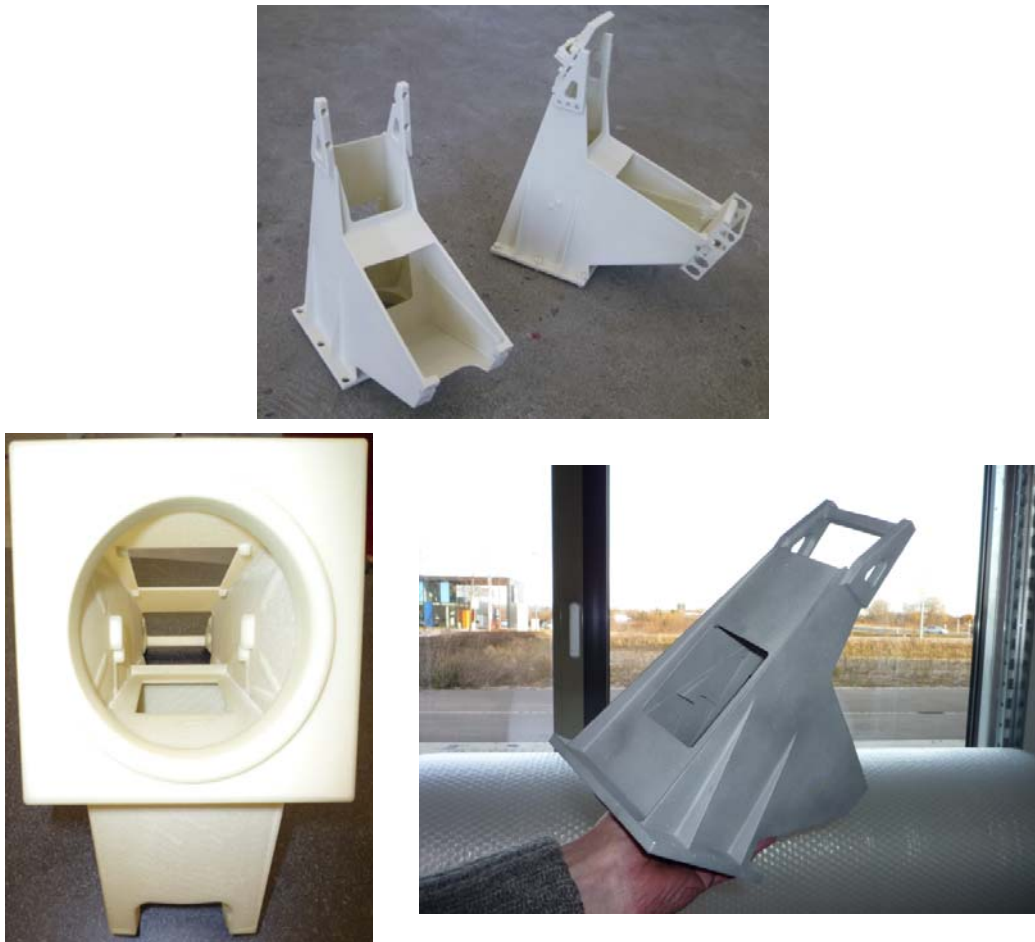
Figure 9. The PMMA part manufactured by 3D-printing (Illustrative models on the top). The Wax infiltrated model is then processed to produce a ceramic mold. Then the chosen metal is casted in the mold (in this case Aluminum G-AlSi10Mg T6). The final result is shown on the bottom right. The remaining steps to complete the part manufacture include the thermal treatment and a conventional machining of some surfaces, which required high accuracy as are used for interfaces
