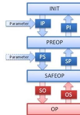
**Figure 4:** TC3 module state machine (source: BECKHOFF website)
