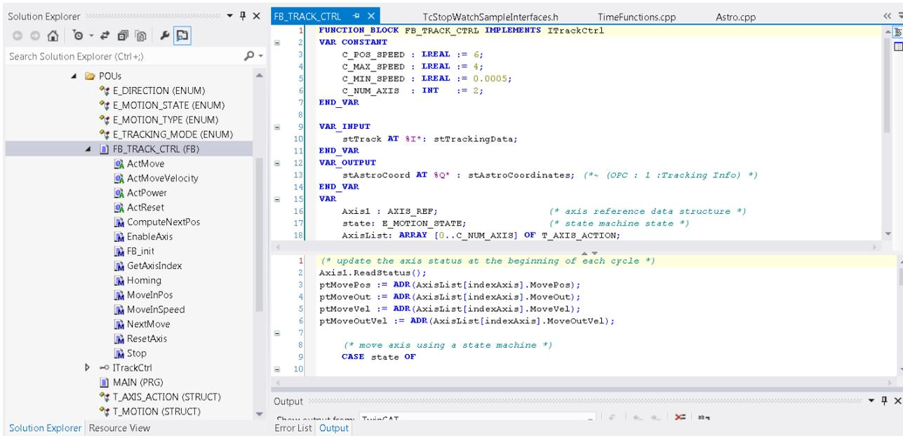
Figure 11: PLC module prototype implementation.
