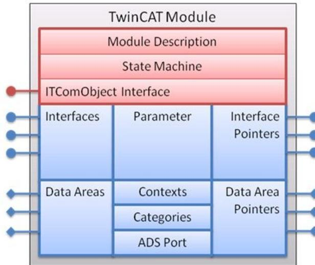
**Figure 3:** Internal structure of a TC3 module (source: BECKHOFF website)
