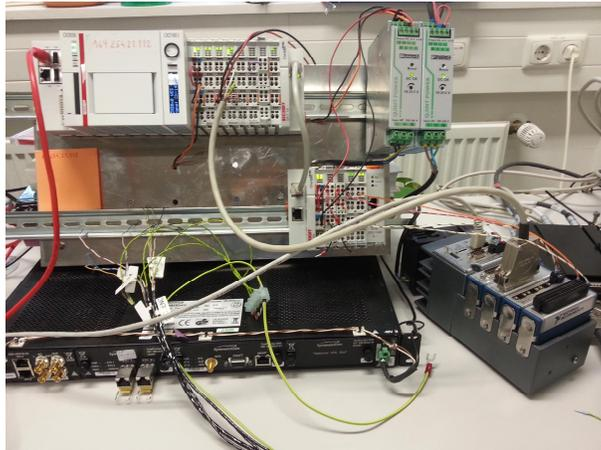
Figure 12: Laboratory setup for the integration of ESTAC on a BECKHOFF PLC.
