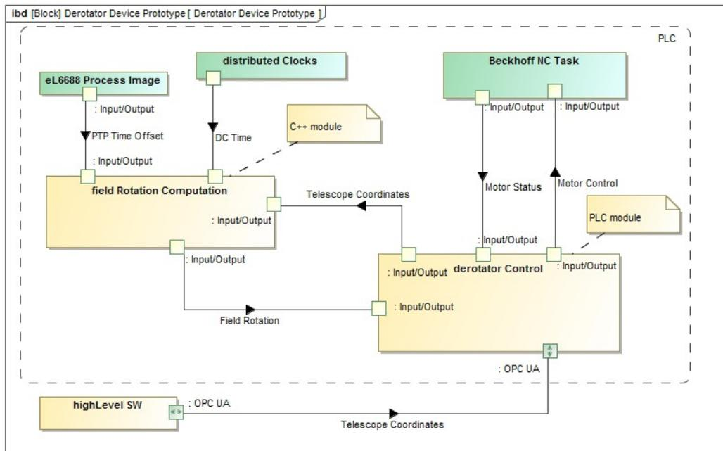
Figure 9: Derotator device architecture (prototype).
