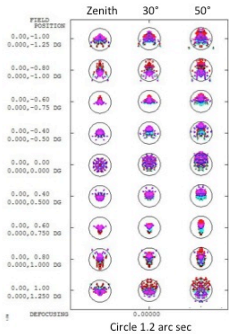
Figure 3: Polychromatic image quality (360-1300 nm) at different locations in the FOV and at different zenith distances.
