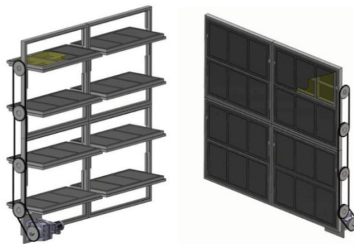
Figure 3.31. Louver design in open and closed configurations.
