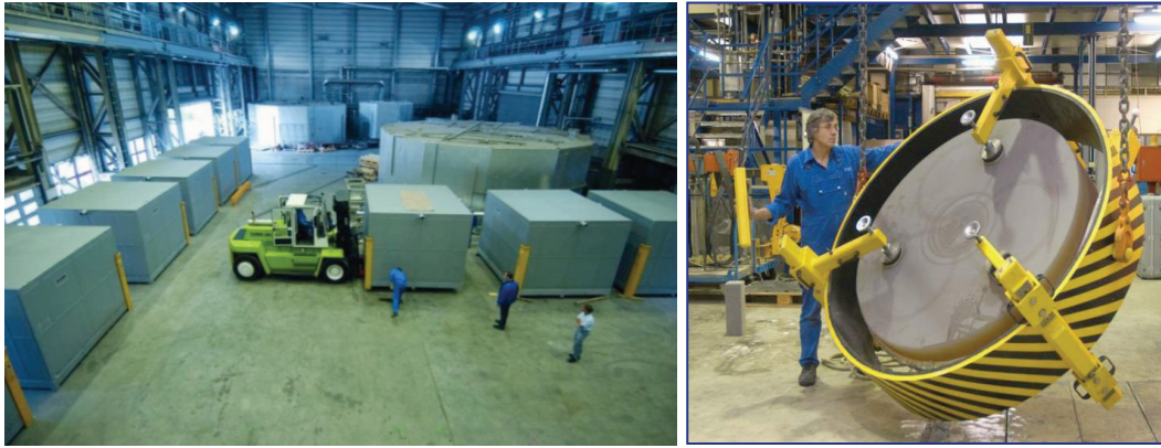
Figure 3.82. Left: Annealing facility at Schott in Mainz. Right: Sample boule.
