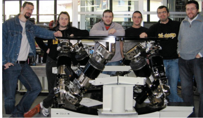
Figure 3.152. M4 mounting structure and positioning system for the Dark Energy CAMera.
