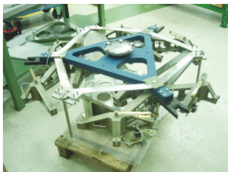
Figure 3.116. Components of the CESA design for the segment support and prototype system.
