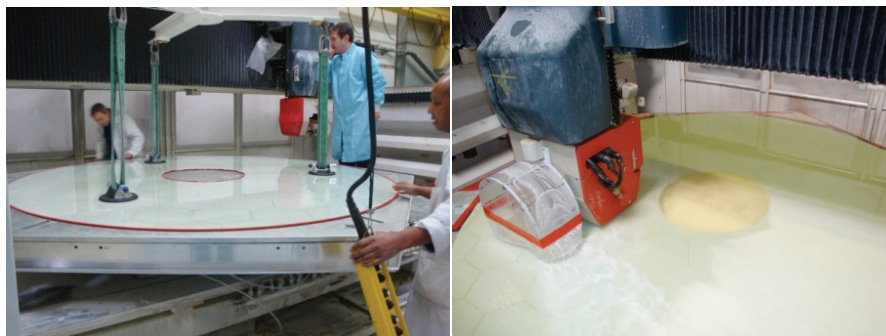
Figure 3.155. The 2.7-metre 2 mm thin shell on the blocking body and in the thinning process.
