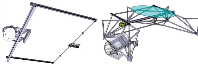
Figure 3.187. Adaptive optics calibration unit trolley and structure supporting the projector.
