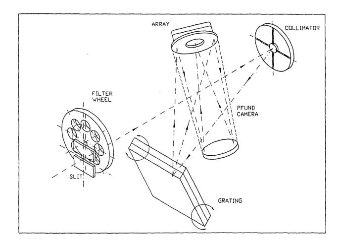
Figure 2.1: Schematic of IRSPEC
