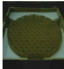
Figure 2.6 [JPG: 419k]. The first VLT M2 Beryllium Mirror in the test laboratory of DASA (Ottobrunn near Munich, Germany), during the determination of its inertia and center of gravity. The mirror is covered by a peelable protective layer. (September 1997).
