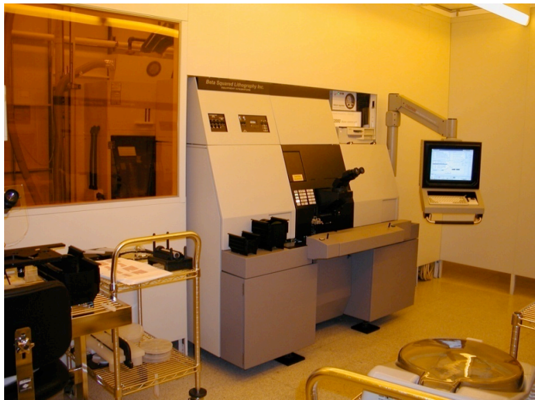
Projection aligner lithography system Beta Squared Lithography (P/E)
