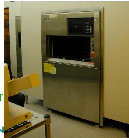
Projection aligner lithography system Beta Squared Lithography (P/E)
