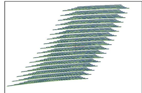
Spectral footprint in higher dispersion mode - 3" slits spaced 25" apart, five orders
