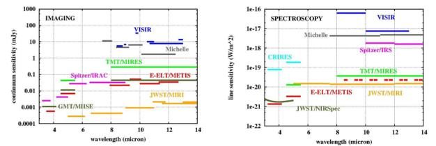
Sensitivity of the imager and IFU-spectrograph of METIS compared to other current and future instruments. Sensitivities are given for a one hour exposure of a pointsource /unresolved line, with 20% overhead and a signal-to-noise of 10. The calculations of these sensitivities are based on an instrument simulator developed by Kendrew et al. (2010)[1].
