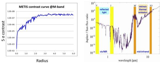
Left: Achievable 5- $\sigma$  radial contrast curves for an A0V star at 10 parsecs observed with METIS at M-band over one hour. Right: Much reduced star-planet contrast in the thermal infrared.
