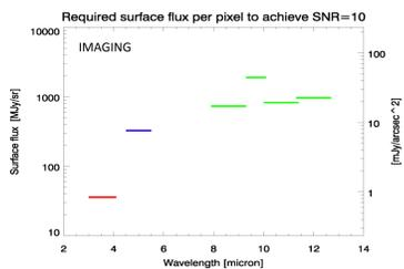
The plot above shows the estimated sensitivities for extended sources in imaging mode on a minimum required flux-per-pixel basis to achieve a S/N=10 in 1 hour on-source integration time for the L, M and N band filters.
