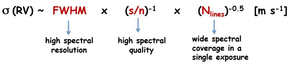
R=100k i.e. FWHM=3x10<sup>3</sup> m s<sup>-1</sup>, s/n~1000,  $N_{lines}$ =1000  $\rightarrow \sigma(RV)$  ~0.1 m s<sup>-1</sup>
