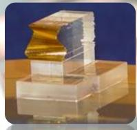
sinfoni uses an image slicer to produce spatially resolved spectroscopic data.
