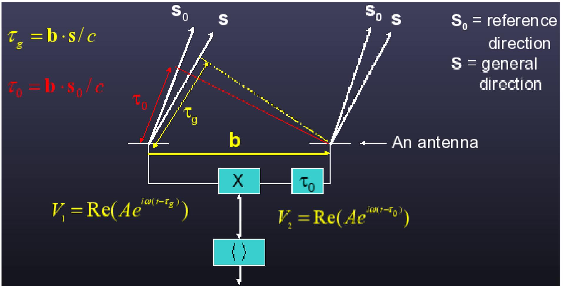
The geometrical delay  $\tau_0$  for the delay tracking centre can be calculated accurately from antenna position + Earth rotation model.
