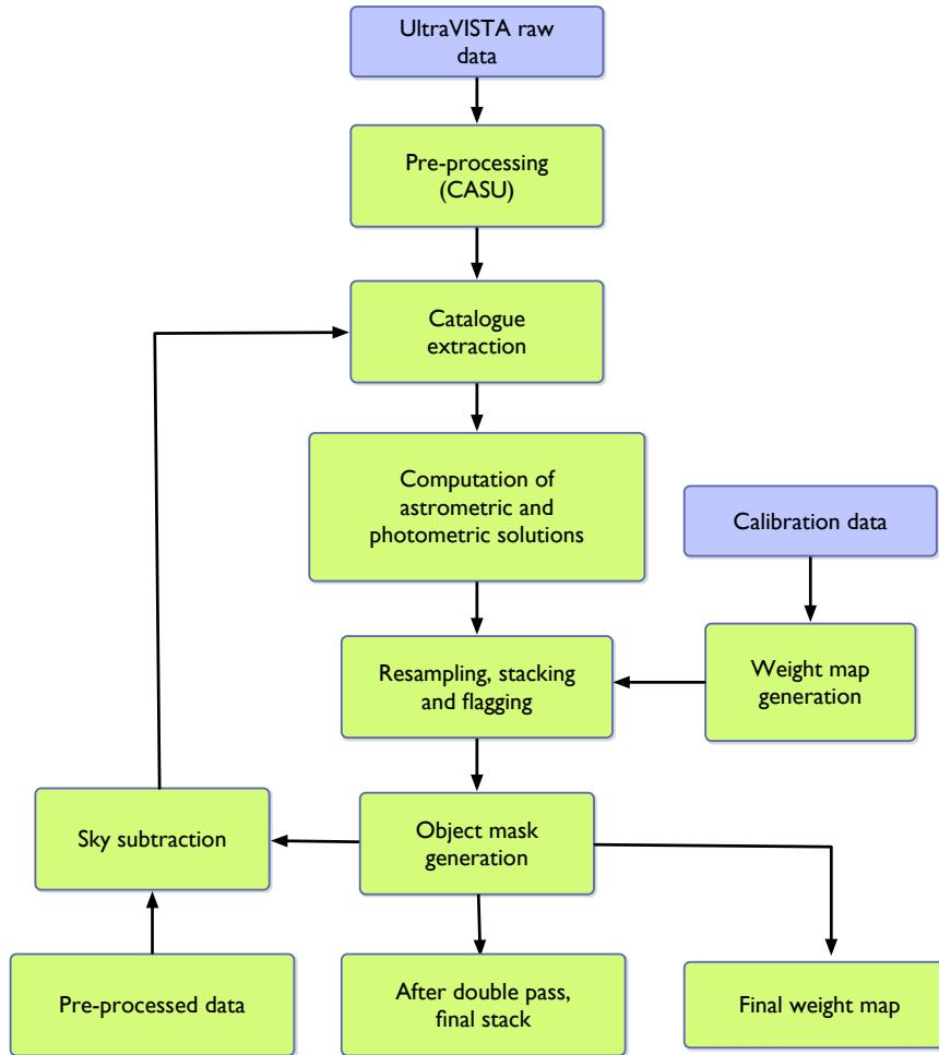
Figure 3: Block diagram of the UltraVISTA extension data processing. Note the double loop in the processing necessary to sky-subtract the images. In addition, in the actual survey data processing, astrometric and photometric computations are made using all available data in all bands. A threshold in seeing, ellipticity and photometric conditions is also normally applied before the final stack.
