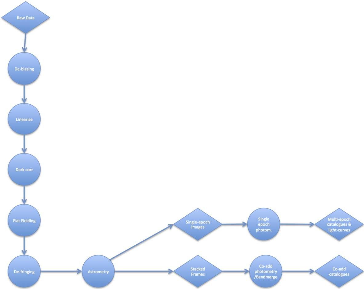
Figure 1: A block diagram synthesizing each step from raw data to the calibrated product is presented.
