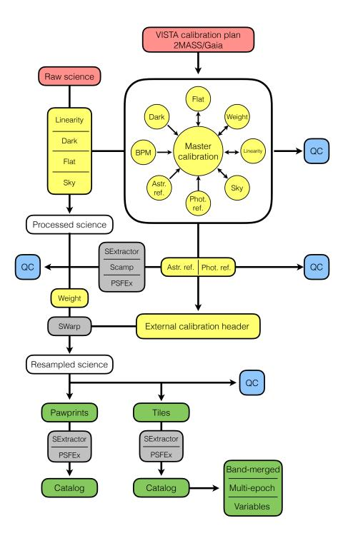
Figure 3: Schematic view of the basic Astropype processing steps. Input data is highlighted in red, calibration steps in yellow, quality control in blue, intermediate products in white, external software in gray, and deliverables in green.
