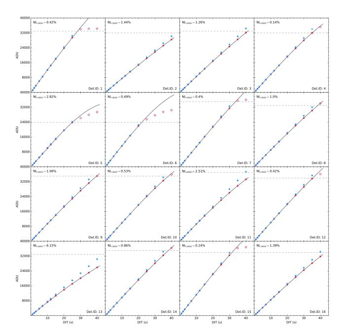
Figure 5: QC unit generated by Astropype to measure non-linearity of the VIRCAM detectors for a randomly selected dome-flat sequence from the VISTA calibration plan.
