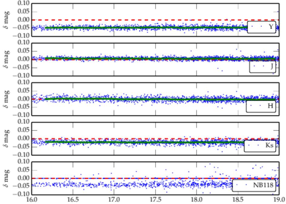
**Figure 2:** Magnitude difference  $\delta$  between  $7.1''$  aperture  $J$ ,  $H$ , and  $K_s$  magnitudes of stars in UltraVISTA DR1 with the corresponding sources in DR2 release. The green line corresponds to a running median computed over 100 objects.
