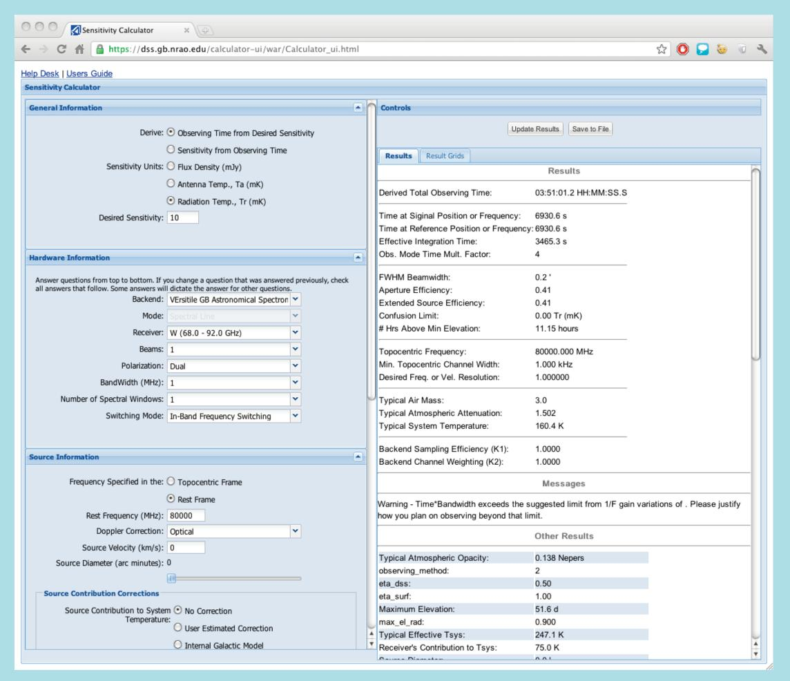
The hardware information section (seen in the figure above) contains all possible hardware configurations supported by the GBT, for which there are currently 8005. The configurations are managed by the science support staff and imported into the DSS database when updates are made. The hardware configuration database design follows a "star pattern", shown below.
