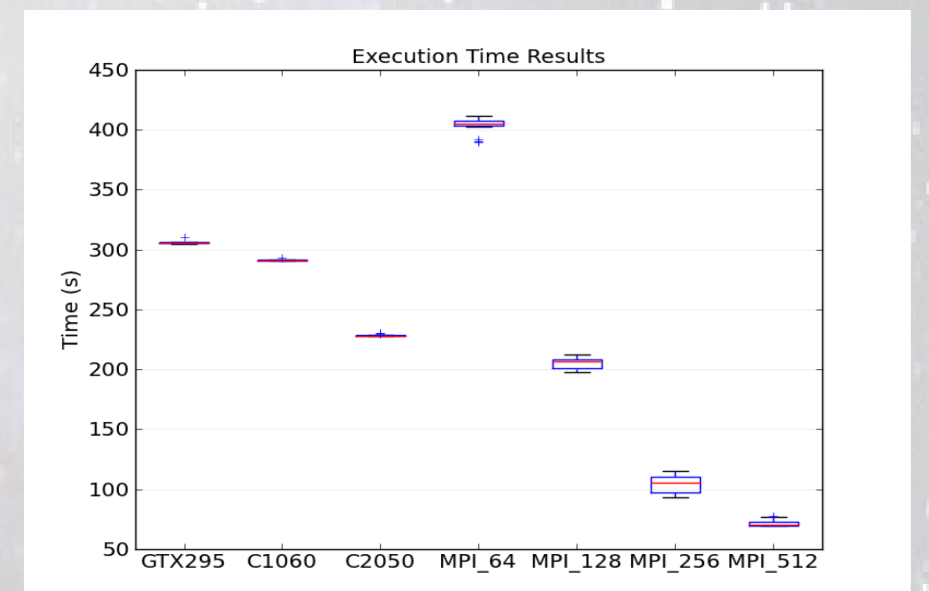
Fig. 2: Comparison between MPI time and different GPUs time.
