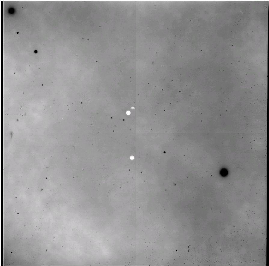
A U band flat field from the 31 st of October, with lamp to LADC reflexion in the middle.
