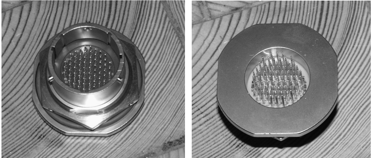
Figure 9: Vacuum connectors that allows to be soldered to be PCB, Hirelco B34222 74000Y-15E-35P-565 N/R
