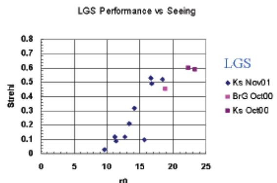
Figure 2: Lick Observatory 3 m telescope results with their experimental LGS-AO. The K-band Strehl ratio vs Fried parameter size,  $r_0$ , is shown. A Fried parameter of 15 cm at 0.5  $\mu\text{m}$  wavelength corresponds to a seeing of 0.7 arc-sec (Courtesy of Don Gavel, Lick Obs.).
