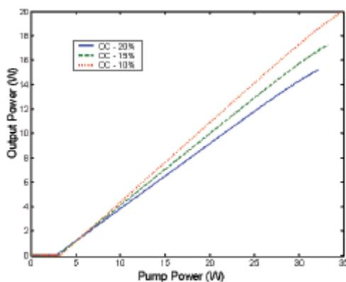
**Figure 6:** Numerical Simulations results for the fibre Raman laser. The 1178 nm output power obtained vs. pump power is shown, for different output couplers. A 10% output coupler will give the best performance of the fibre laser. 1121 nm pump powers up to 100W are now commercially available.
