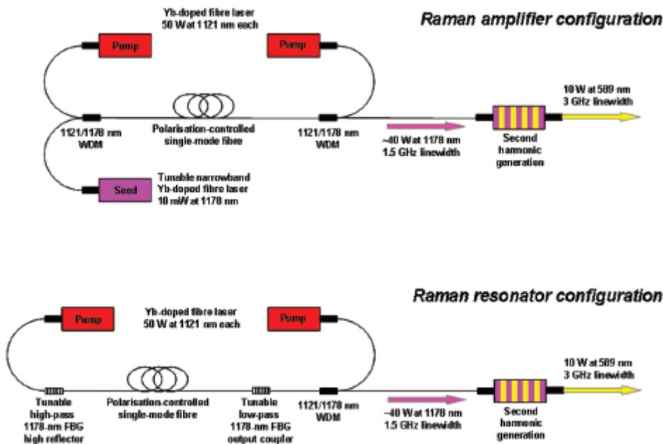
**Figure 4:** The fibre Raman laser at 589 nm is obtained by frequency doubling a laser at 1178 nm via a second harmonic generation crystal. The 1178 nm wavelength is obtained as the first Stokes of a Stimulated Raman Scattering process. The two configurations of amplifier (upper drawing) and resonator (lower drawing) are being breadboarded.
