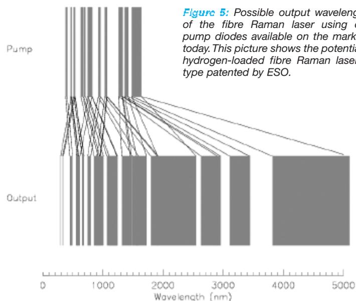
**Figure 5:** Possible output wavelengths out of the fibre Raman laser using different pump diodes available on the market as of today. This picture shows the potential of a hydrogen-loaded fibre Raman laser of the type patented by ESO.
