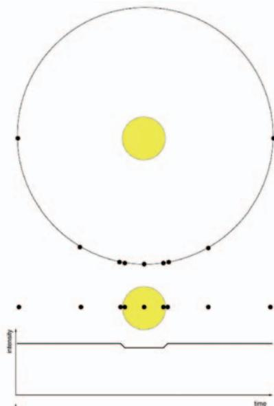
Variations in stellar brightness and velocity, caused by an orbiting exoplanet that transits the disk of its central star. Consecutive positions of the planet in its (circular) orbit are marked by black dots, with the motion from left to right.
