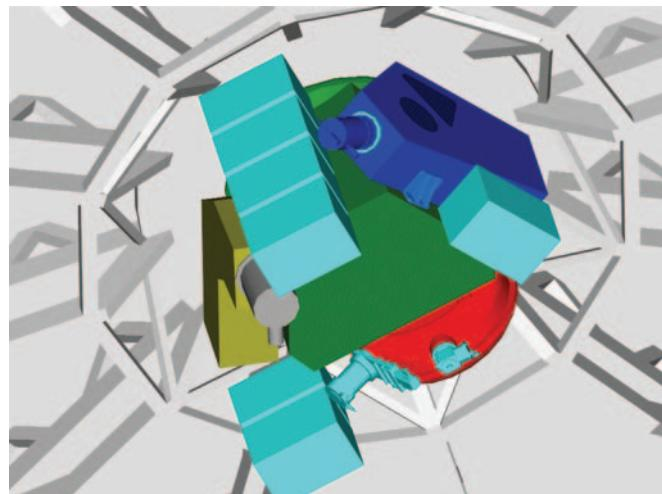
**Figure 4:** A CAD view of X-shooter attached to the Cassegrain focus of the telescope. While this opto-mechanical layout is likely to be substantially modified in the design of an optimized structure, it conveys the instrument concept based on the parallel operation of three arms operating in the UV, Visual-red and *J-H* bands.
