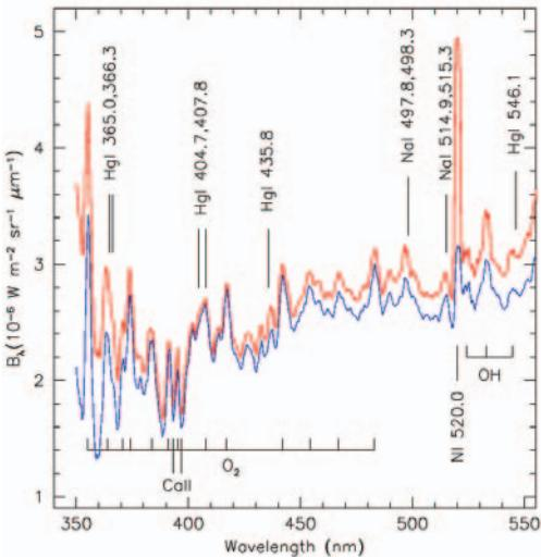
**Figure 5 :** Night sky spectrum obtained at Paranal on February 25, 2002 at 04:53 UT (blue line). Marked are the expected positions for the most common lines produced by artificial scattered light (upper ticks) and natural atmospheric features (lower ticks). The blue line traces part of the spectrum taken during the same night at 02:39 UT.
