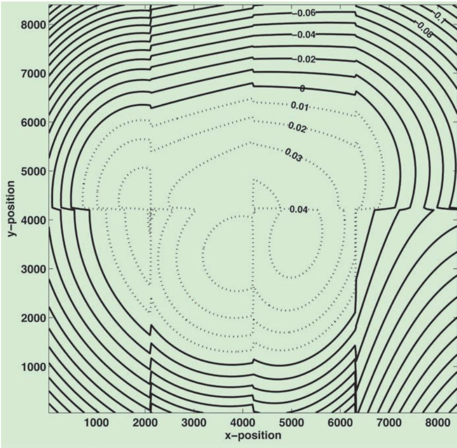
**Figure 2:** Best-fit second-order calibration map after removal of the mean offsets that arose from different flatfield scale factors. The map for the R-band is on the left, the right panel shows the correction map for the V filter. Contours are separated by 0.01 mag. Near the centre of the camera, stars are measured fainter than near the edge.
