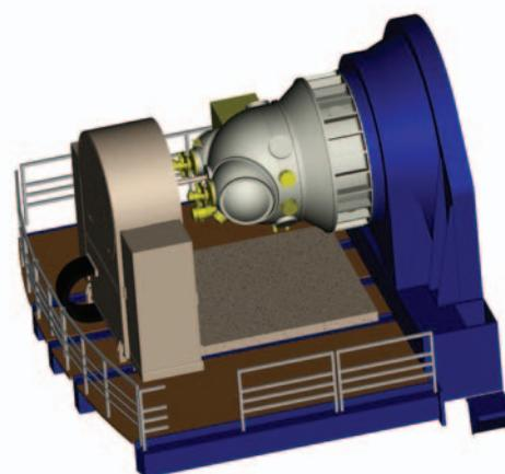
**Figure 2:** HAWK-I installed at a Nasmyth focus. The large port on this side of the vacuum vessel allows easy access to the detector mosaic and the filter wheels without dismounting the instrument.
