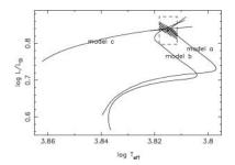
Figure 11: Evolutionary tracks in the Hertzsprung-Russel diagram of three models of Procyon A. The dashed rectangle delimits the classical uncertainty domain for luminosity and effective temperature, while the hatched area delimits the much reduced uncertainty when considering the interferometric radius. Model a is the most probable and indicates an age of 2.3 Gyr. From Kervella et al. (2004f).
