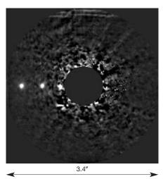
Figure 4: Final SDI image (double filtered) derived from real data which was used to derive the detection limits shown in Figure 3. The three artificial companions at 0.5", 1" and 1.5" with Δmag = 9.5 (5σ detection at 0.5") are clearly visible.
