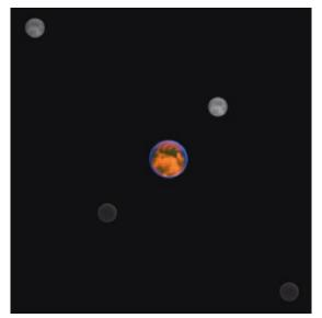
Figure 5: Titan imaged with SDI. The picture shows Titan imaged through the 4 channels of the SDI camera. Obviously, Titan appears very faint and featureless when imaged inside the methane band in the barely visible lower two images. The central color image is the difference between the out- and in-band images and has been added to the picture afterwards.
