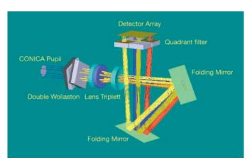
Figure 2: SDI optical concept. A double Wollaston prism splits the beam into four which are imaged through different filters located on the either side of the *H*-band methane feature at 1.62 μm.
