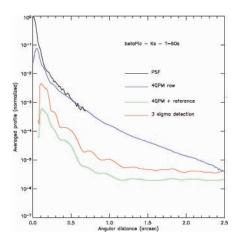
Figure 6: Radial detectivity of the 4QPM. The achievable 3σ detectivity is 10<sup>-4</sup> (10 mag) at 0.5" and 10<sup>-5</sup> (12.5 mag) at 1". Stellar residuals, i.e., the quality of the PSF reference subtraction, dominate at short angular distance, while sky and detector noise dominate at larger angular separations for this star magnitude and exposure time (courtesy Anthony Boccaletti).
