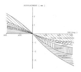
Figure 1: M1/M2 relative displacement with Declination.
