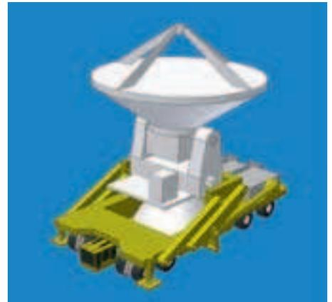
Figure 4. Transporter design with hydrostatically driven wheels.
