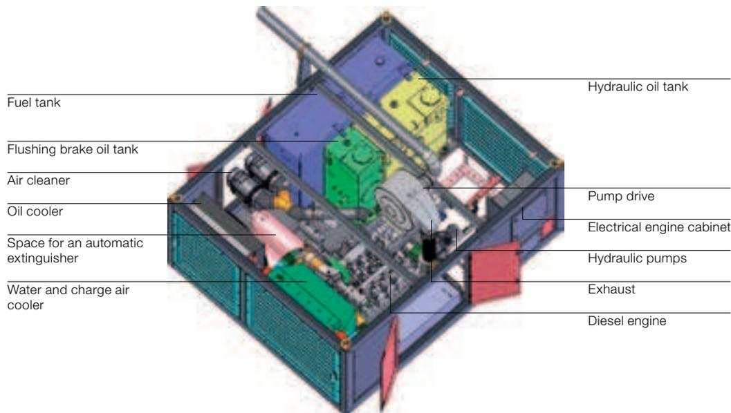
**Figure 9.** One of two installed engine units. Each unit is self-sufficient and can be quickly changed in case of problems. One unit is capable of moving the transporter in cases of emergency. (Figure: Scheuerle Fahrzeug GmbH)
