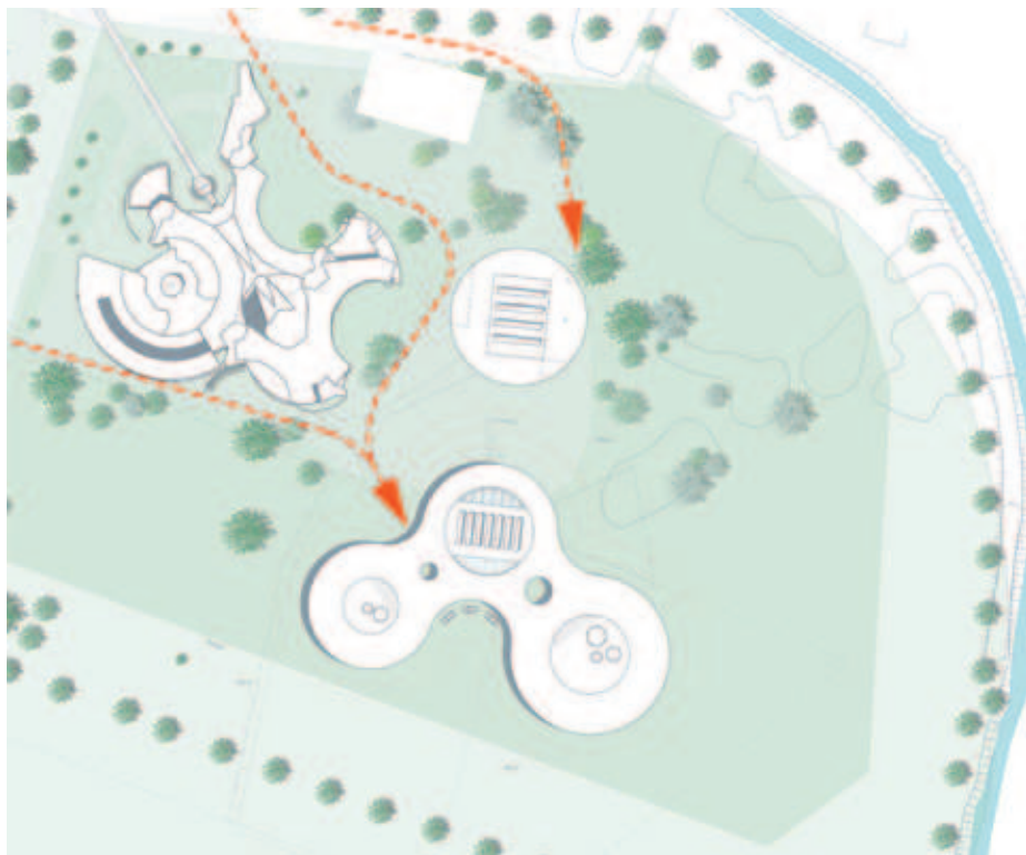
Figure 3. Ground plan of the Auer + Weber design for the ESO Headquarters. The single circular building to the north is the technical building.
