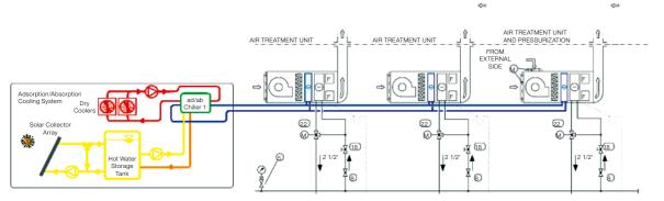
Figure 3. A solar-powered cooling circuit for one Unit Telescope is shown. See text for explanation of the various elements. The solar circuit is shown in yellow; ab(d)sorption cooler in green; dry cooler (red); cooled media delivery (blue) for three air-handling units at the telescopes (only one shown).
