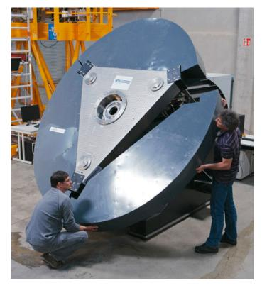
unit has been manufactured for the tip-tilt M5 mirror (see Figure 4).
