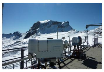
Figure 1a. On 19 September 2011 almost half a metre of snow had to be cleared on the terrace of the UFS Schneefernerhaus before the LHATPRO radiometer could be set up for its test period in Europe.
