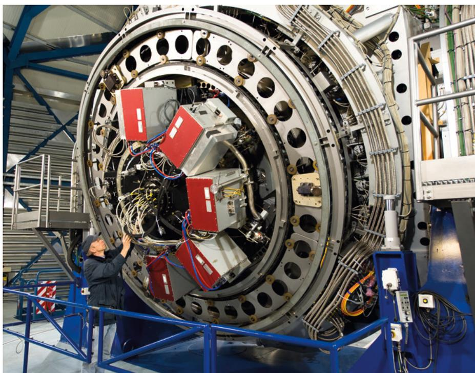
View of the Cassegrain focus of VISTA housing the VIRCAM camera. VIRCAM consists of 16 2048 square Raytheon VIRGO HgCdTe 0.84–2.5  $\mu\text{m}$  detectors covering a field of  $45 \times 45$  arc-minutes (with inter-detector gaps). This image shows Paranal engineer Gerhard Hüdepohl checking VIRCAM.
