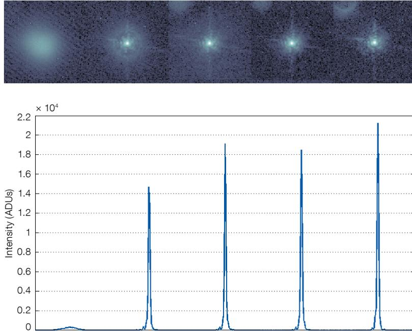
Figure 7. Long-exposure *H*-band images (top) and their horizontal cuts (bottom) recorded (from left to right): in open loop turbulence, in closed loop on turbulence with 150, 550 and 950 modes controlled, and in closed loop on the calibration fibre (rightmost image).
