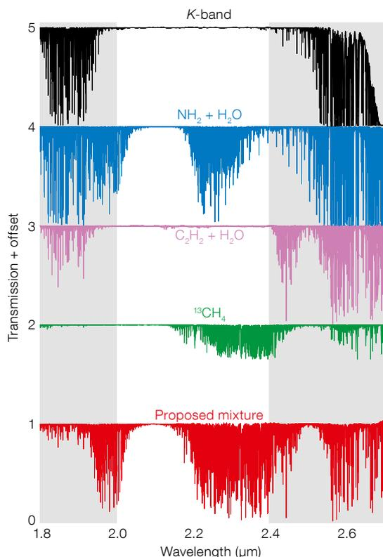
**Figure 4.** Transmission spectra of the gases for the CRIRES+ gas cell in the *K*-band are shown. The top panel plots the telluric (water) contribution, while the second to fourth panels show measurements of the individual species. The bottom spectrum presents the measured compound gas cell, which is a mixture of the above.
