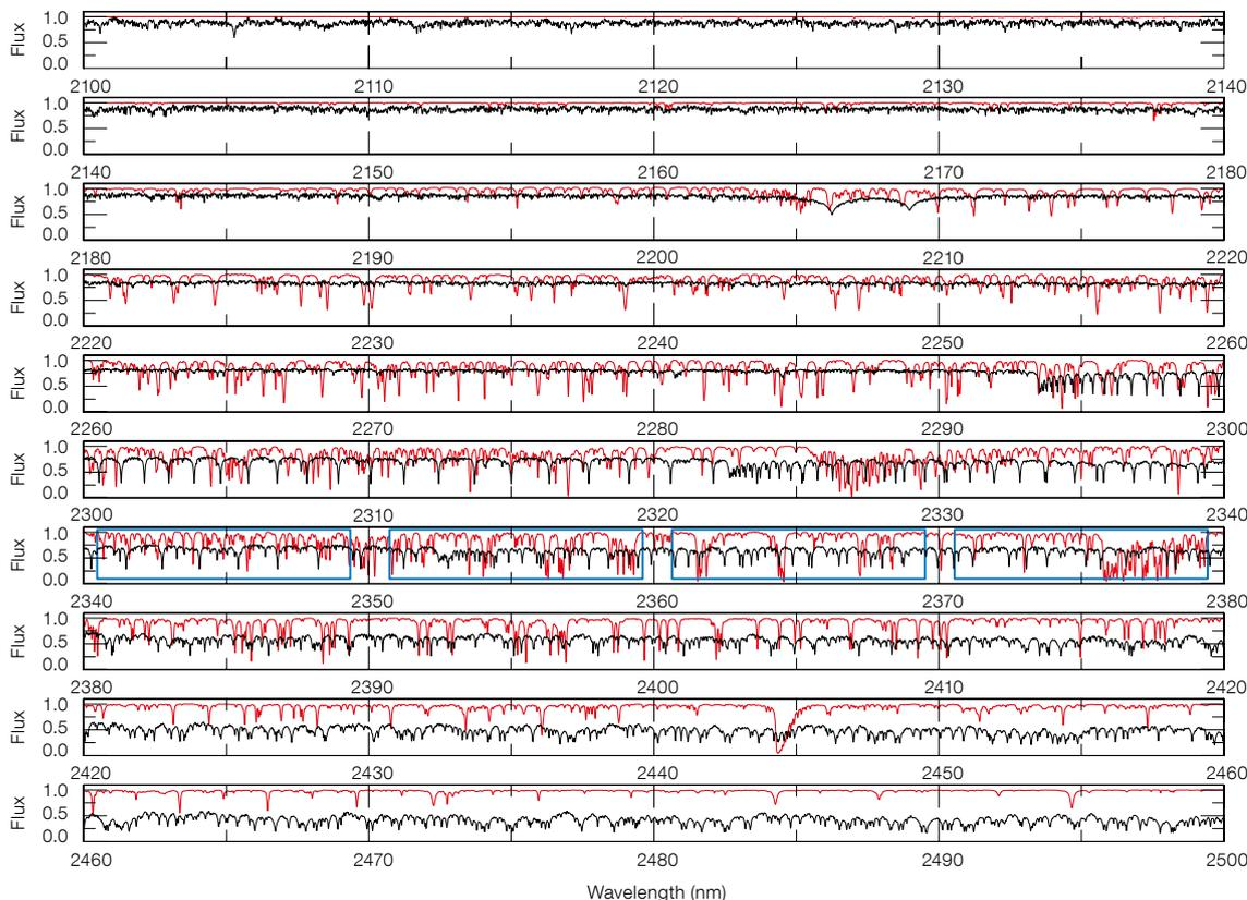
Figure 1. The wavelength coverage of the current CRILES (blue boxes correspond to the four Aladdin detectors currently installed) in the K-band compared to the expected coverage of a single exposure from CRILES+. The black line shows the spectrum of an M4 dwarf star ( $\sim 0.15 M_{\odot}$ ) and the light brown line is a laboratory spectrum of the first gas cell prototype being developed at the University of Göttingen.
