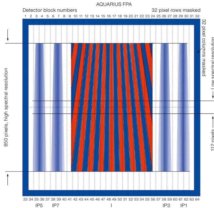
**Figure 3.** The layout of the interferometric pattern (central detector blocks, dispersion direction vertical) and the four photometric signals (outer detector blocks) on the AQUARIUS detector is shown for the SiPhot mode in *N*-band with medium spectral resolution dispersion.
