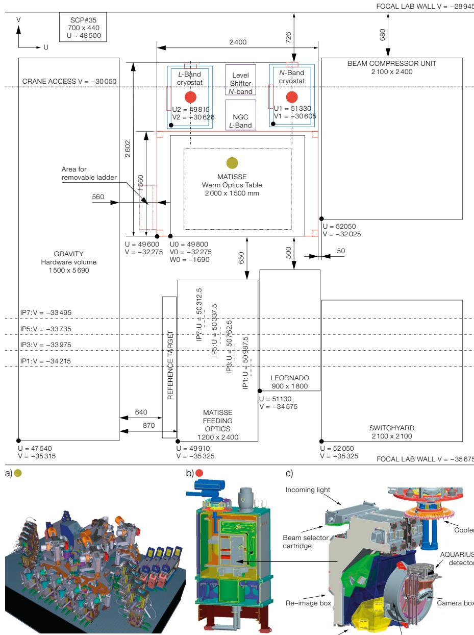
**Figure 4.** The future location of MATISSE in the VLTI laboratory is sketched. The warm optics table and the two cryostats are viewed from above. This location is currently used by MIDI. Sub-figure (a) shows the MATISSE warm optics bench with its optical
