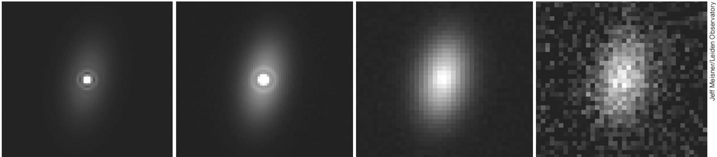
**Figure 2.** Using a model of a star surrounded by cooler circumstellar material, the METIS simulator predicts detector images using four different camera filters (from left to right) *L*-band (3.8  $\mu\text{m}$ ), *M*-band (5  $\mu\text{m}$ ), *N*-band (10.7  $\mu\text{m}$ ), and *Q*-band (17.7  $\mu\text{m}$ ). At shorter wavelengths the hotter star dominates; at longer wavelengths the nebulous component is brighter and the instrument sensitivity decreases.
