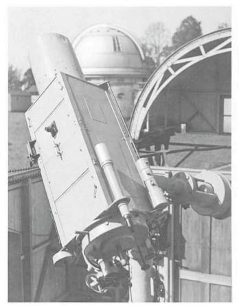
Fig. 2: The Original Schmidt Telescope at the Hamburg Observatory; f/1.75, 15° field.
