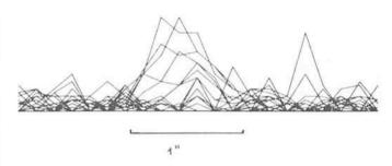
Fig. 2: A scan through one of the images in figure 1, made with the PDS microdensitometer at the Lund Observatory through a  $10 \times 10$  micron square aperture.
